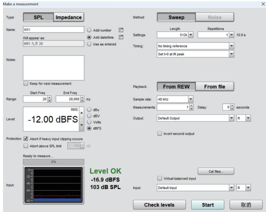
The level can also be inspected in this interface, as shown above, the ‘Level OK’ means the level meets the requirements. Next, click ‘Start’ , REW will begin the measurement and get a set of room curves. We name this set as MR1. As it is shown below, 1/3 smoothing has been applied.
