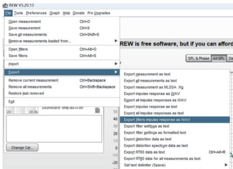
Because we only measure the right channel, please select mono audio and use 32-bit floating-point data type for saving. The most important thing is that the sampling rate must be set to 48000, consistent with the sampling rate used in the data processing of the DMP-A8 DSP. Click OK to save it as a WAV file, and we name it MR1-filters. Copy the file to a USB drive for backup.
