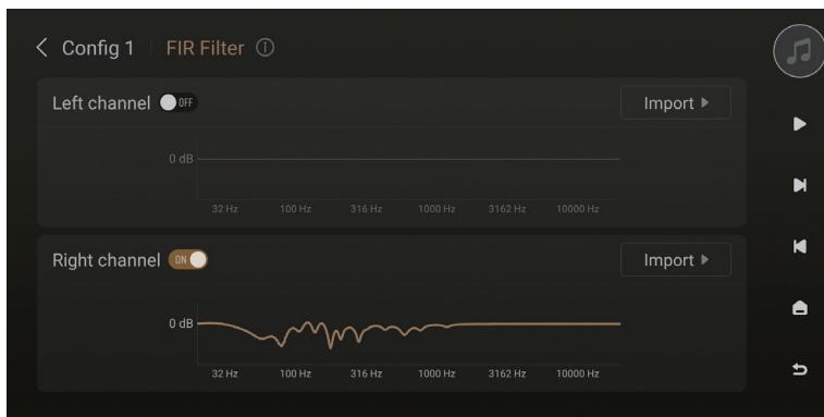
Next, validate whether the FIR filter is functioning properly. Remember to turn on the switch for the right channel in the FIR filter interface, and also, make sure to turn on the input source DSP switch.
