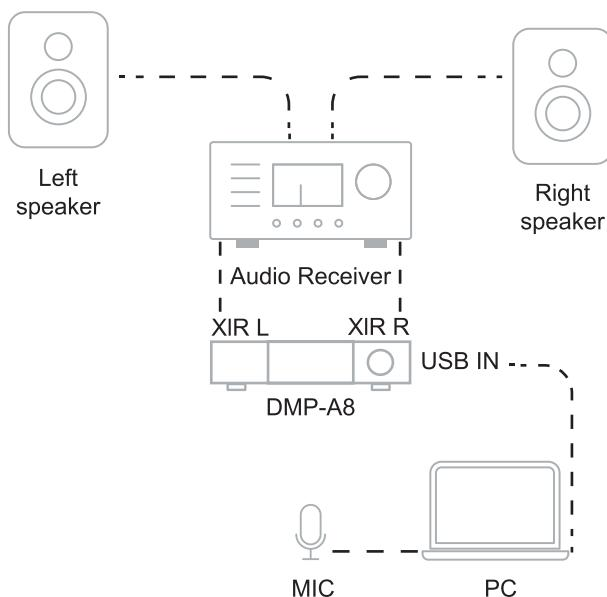
First, set the DMP-A8 as Soundcard, connecting your PC to DMP-A8 via USB cable.
