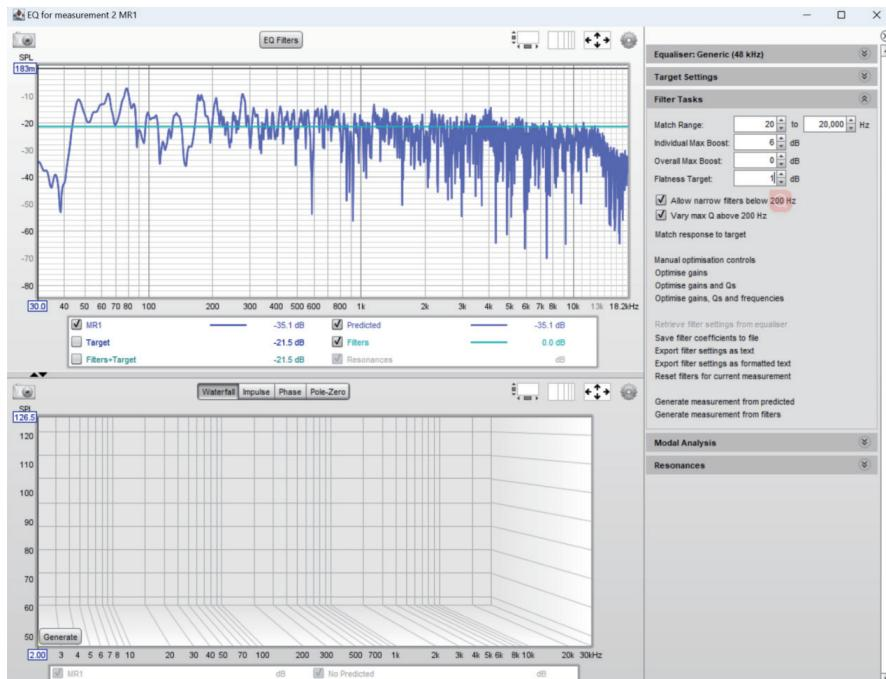
After the above parameters are set, you can click 'Match Response to Target' to initiate the automatic filter allocation and adjustment process in REW, generating the correction EQ and response.
