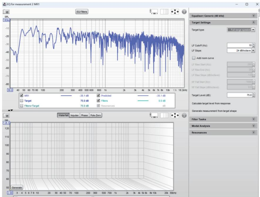
If you not sure about the Target Level. Click on ‘Calculate target level from response’ to calculate automatically.
