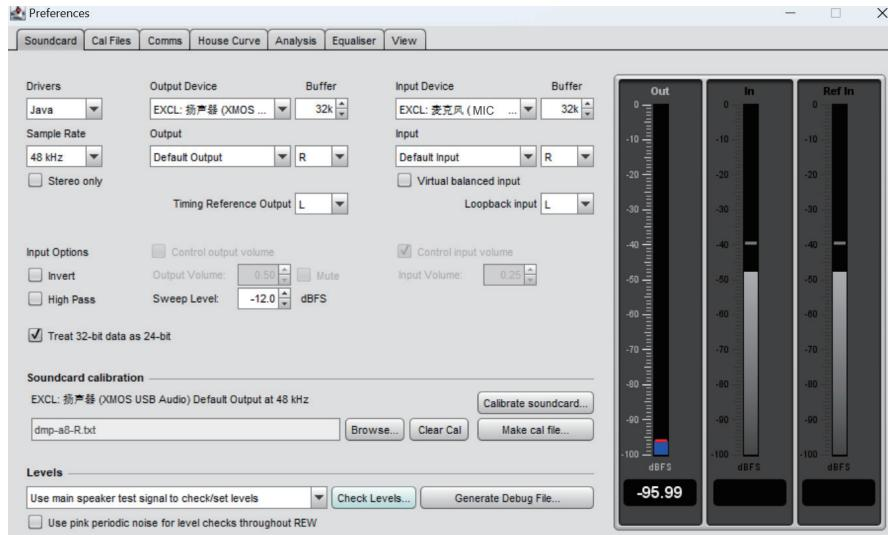
Before measuring, click on 'Check Levels' to inspect the input level and ensure it meets the requirements of REW. If the level is too low, you can increase the volume of DMP-A8, or decrease the volume if the level is too high. If your Soundcard is not calibrated, click on 'Calibrate Soundcard' and follow the prompts at the bottom of the interface to measure the Soundcard.
