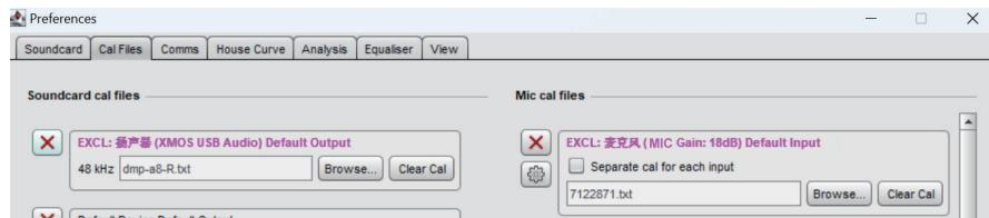
After launching REW, click the Preferences option on the top right corner to enter the configuration interface. You will see the Soundcard interface by default, please set the input and output device for the sound. In this test, we choose DMP-A8(the drive name of DMP-A8 is shown in the picture as below) and UMIK-1. Also, please select the measurement channel, in this example the measurement is done on the right channel.
