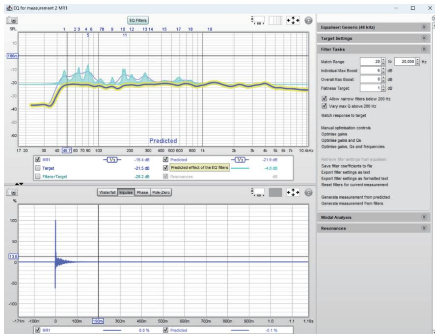
We have completed the calibration for one measurement at this point. If you are not satisfied with the calibration results, you can adjust by taking multiple sets of measurements and averaging them, as well as adjusting the target levels and filter parameters until the desired results are achieved.
