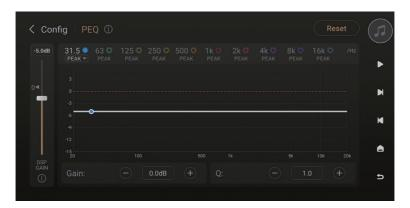
The PEQ can be customized according to your needs, and different filters can be set for each frequency band.
