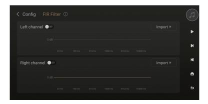
The FIR Filter design only supports importing files. Different values can be set for left and right channels. The supported file types are bin and WAV formats.
